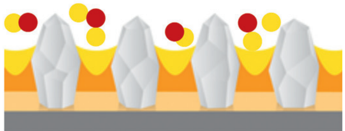
The anti-loading system (yellow) binds sanding dust, resulting in a significantly longer work life.
