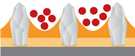
Without anti-loading system – Abrasive dust particles load up the disc. The removal rate deteriorates.
